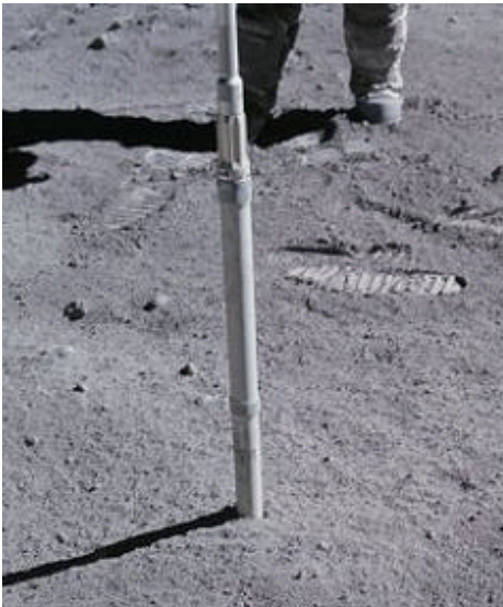
Apollo 16 astronaut Charlie Duke (feet shown) drives a core sample tube into the lunar regolith.
